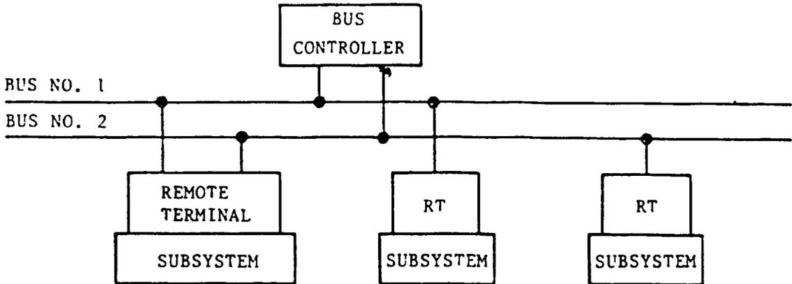
FIGURE 11. Illustration of possible redundancy.
