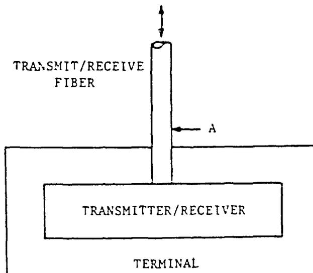
\*FIGURE 10. Data bus interface using a single transmit and receive fiber.
