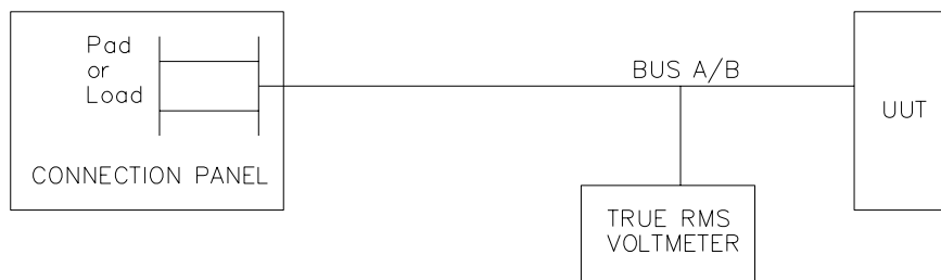
Figure 1. Output Noise Test Configuration
