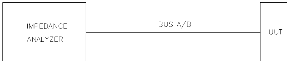
Figure 3. Input Impedance Test Configuration
